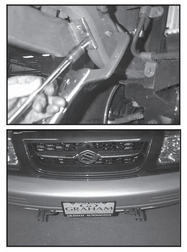
Install self-threading bolts at this time, and tighten all previously mentioned hardware to proper torque specifications. Remove C-clamps We require that "LOCTITE. Blue" be used on all bolts.
