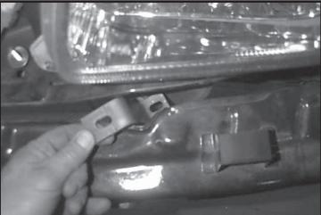
Remove top bumper bolt on each side and install brace with 8mm x 1.25 x 25mm bolt, 8mm lockwasher, and 8mm fender washer. Secure bottom of brace to frame mount using 3/8" x 1-1/4" bolt, 3/8" lockwasher, 3/8" flatwasher, and 3/8" hex nut. We require that "LOCTITE. Blue" be used on all bolts.
