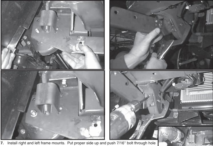
7. Install right and left frame mounts. Put proper side up and push 7/16" bolt through hole and start 7/16" lockwasher, and hex nut. Start 10mm x 1.25 punch lock nut over factory stud. Push mount up so angle is flat on front of frame, and clamp with C-clamp. Snug previously mentioned fasteners. Drill 5/16" holes through frame using mount as a template (three on each mount).
