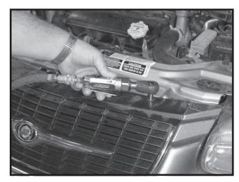
Open hood and remove six screws from top of grill and facia.
