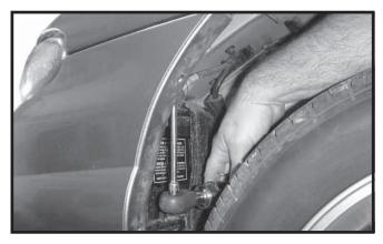
**5.** Remove two nuts holding facia to fender on each side by going through wheel well opening.
