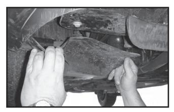
4. On passenger side, loosen front portion of wheel well extension, two plastic push fasteners, and remove approximately four more plastic push fasteners from inside of wheel well. This is done to gain access to nuts holding facia.
