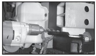
**10.** Center punch all eight holes (four on each side) and drill 3/8" holes through frame lip, using base plate as template.
