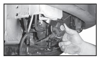
Bend horn bracket to clear base plate when installed.
