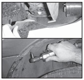
3. Remove plastic wheel well extension, two plastic push fasteners. Remove front portion of driver's side wheel well, held on by four screws.
