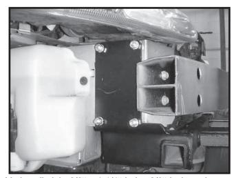
11. Install eight 3/8" x 1-1/4" bolts, 3/8" lock washers, and 3/8" hex nuts. Install bolts from inside outwards. We require that "LOCTITE. Blue" be used on all bolts.
