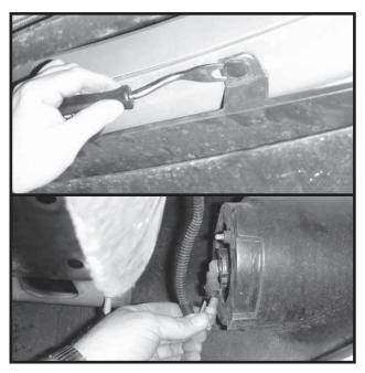
**6.** Remove two plastic push fasteners from bottom side of bumper and unplug fog light.
