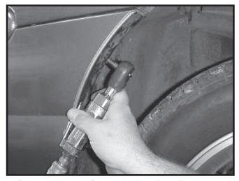
2. Remove screws from wheel well to facia on each side.
