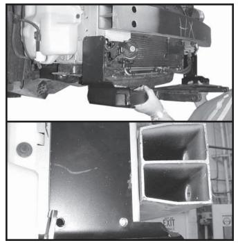
**9.** Slide base plate up from bottom and line up tight against front frame bracket as shown in picture. Clamp in place.
