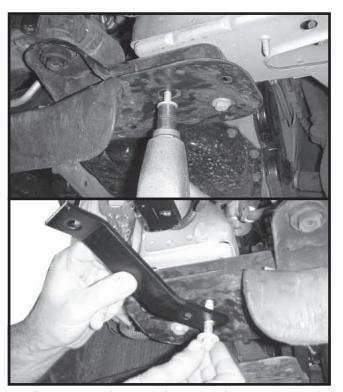
12. Remove one front sub-frame bolt from each side, for bottom brace (see picture). Install long end of brace and refasten long sub-frame bolt. On other end of brace, use 1/2" x 1-1/4" bolt, 1/2" lock washer, and 1/2" hex nut through brace and base plate. Tighten these bolts. Do this on both sides.
