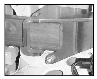
10. Install 3/8" x 1" bolt and flat washer from inside out on previously drilled 3/8" holes on front of vehicle and through base plate. Use 3/8" lock washer and 3/8" hex nut on bolts. Snug this bolt, then tighten 1/2" x 3-1/2" bolts and then go back and tighten the 3/8" x 1" bolts. NOTE: Sides of base plate that go down the side of frame should be straight, if not, adjust and retighten. Also, the previously drilled 3/8" holes may have to be re-drilled or reamed out, using Base plate as template.
