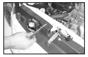
1. Open hood and remove four plastic push fasteners.
