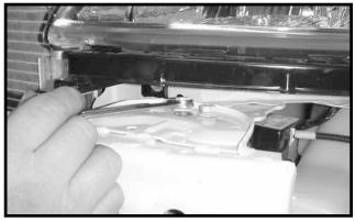
Remove six bolts that hold bumper on, four on the top side and two underneath. Set bumper aside temporarily.
