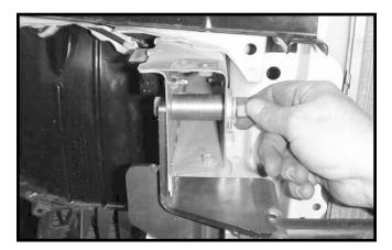
9. With an assistant, slide base plate on frame and install 1/2" x 3-1/2" bolt through base plate and previously installed spacer bushing. On inside of frame, use heavy frame washer, 1/2" lock washer, and 1/2" hex nut. Do not tighten. NOTE: Use LOCTITE® Blue on all bolt threads.
