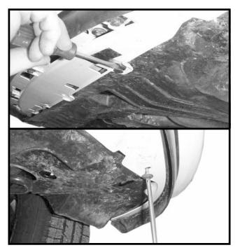
3. Remove six plastic push fasteners from bottom side of facia and one screw from each side that attaches to wheel well extension.
