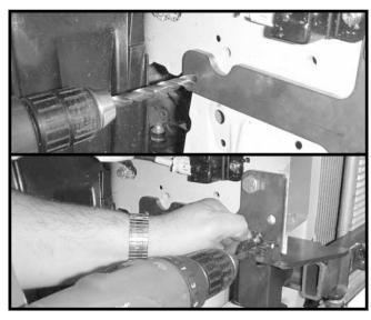
**11.** Drill 3/8" holes, two on each side, through sides of base plate as shown in pictures. Use 3/8" x 1" bolts, 3/8" lock washers, and 3/8" hex nuts. Tighten these bolts.
