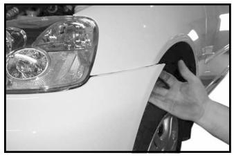
**4.** Pull facia straight out on each side by fender and carefully pull facia off.
