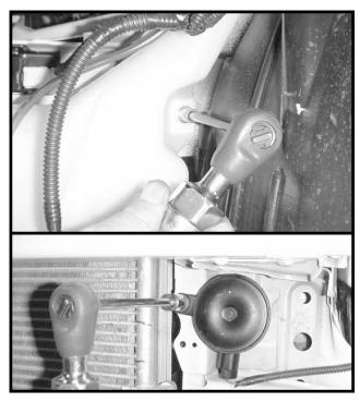
Remove three bolts that hold windshield washer tank and also remove bolt that holds horn and let horn hang.
