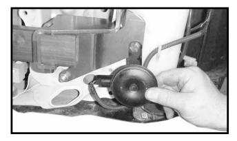
**14.** Reinstall horn with 5/16" x 1" bolt, 5/16" lock washer, and 5/16" hex nut through hole provided in base plate gusset.
