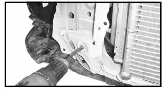
7. Drill out two holes on front of vehicle, one on each side, with 3/8" drill bit. (See picture)
