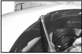
**2.** Remove one screw from each side, facia to fender.
