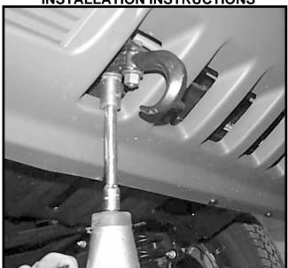
Remove both tow hooks, bolts wll be used for base plate installation, hex nuts will not be used.
