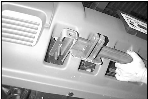
**3.** Before tightening, tow hooks must be pulled outward, for safety cable hook clearance.
