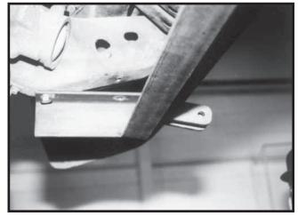
Install base plate with rear bolts snug so front ears touch Air dam/Valance. NOTE: Some bolts may need to be put back in so it is stable for marking and cutting of slots.
