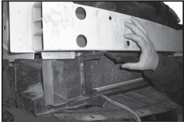
8. Remove plastic filler panel on each side by removing all plastic push fasteners, set panel aside for later notching and reinstallation.
