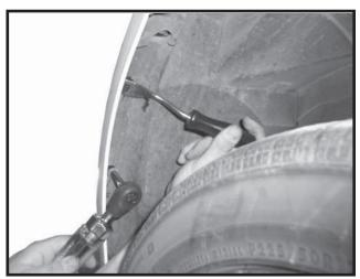
Remove three plastic push fasteners and one screw from wheel well on each side.
