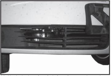
**14.** Notch plastic on front facia for pull ears as shown above. Reinstall facia, plastic filler panels and all hardware. Install horn with longer supplied metric bolt, washer, and lockwasher.
