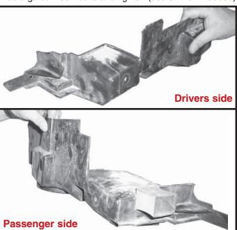
**13.** Notch plastic filler panel as shown in picture on each side and replace.
