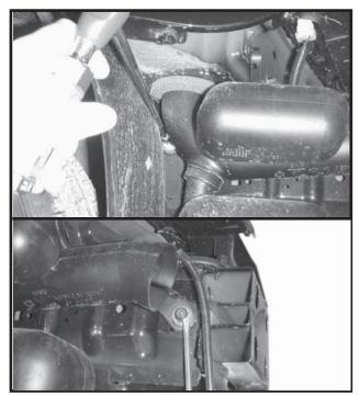
7. Remove air intake on passenger side, by removing one bolt and two plastic push fasteners.
