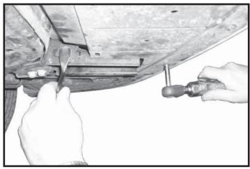
3. Remove plastic filler panel from under facia by removing five screws and two plastic push fasteners.
