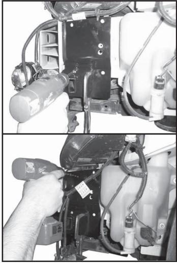
11. Drill bottom two 3/8" holes (on each side) insert bolts and tighten, drill top two 3/8" holes (on each side) place spacer bushings on each as shown on front cover with the longer spacers on the drivers side and the shorter spacers on the passenger side. NOTE: Use Blue LOCTITE. on threads and tighten bolts according to bolt chart on front page.
