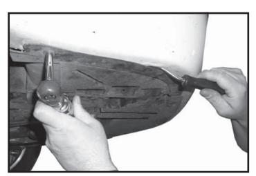
**5.** Remove four plastic push fasteners and one screw from filler panel on each side.
