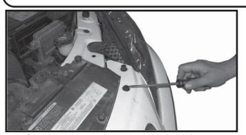
1. Open hood and remove six plastic push fasteners.
