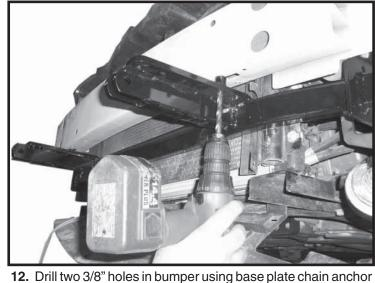
Drill two 3/8" holes in bumper using base plate chain anchor as a guide insert bolts and tighten (use shims if needed).
