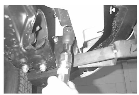
2. Attach right and left mounting bracket with two previously existing bolts on each side.
