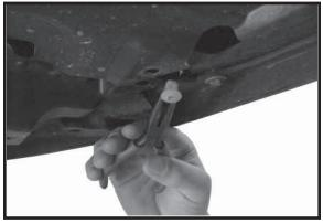
**4.** Remove two plastic screw holders from bottom of facia. Unplug fog lights and clearance lights if equipped.
