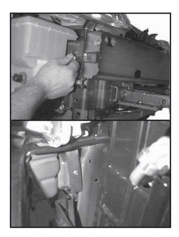
**11.** Install 3/8" x 3-1/2" bolt, 3/8" lock washer, and install through base plate frame, and thread into threaded nut plate on inside of frame. Do not tighten yet.
