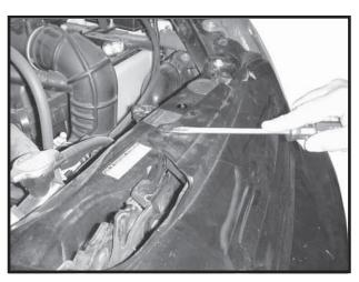
Open hood and remove center grill, four plastic push fasteners and remove.
