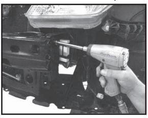
7. On driver's side, remove two bolts holding tow eye bracket, these bolts will be reused, bracket will not. Also, temporarily remove two screws from ceramic box and let hang.
