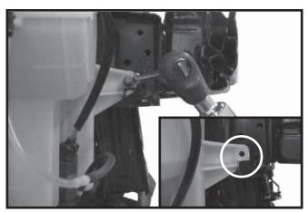
**10.** Remove one bolt in washer tank (washer tank bracket will need to be notched for clearance of baseplate).
