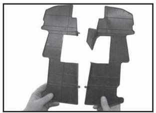
19. Notch plastic shields and reinstall.
