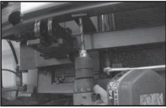
**16.** Drill 3/8" hole through bottom of bumper, using base-plate as template. This is located under bumper on passenger's side.
