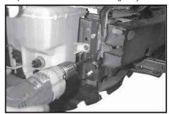
**15.** Next, drill 3/8" hole, using baseplate as template, through flange on vehicle. Install 3/8" x 1" bolt, 3/8" lock washer, and 3/8" hex nut through drilled hole. Tighten all bolts before proceeding. **NOTE:** Use bolt torque chart on front.
