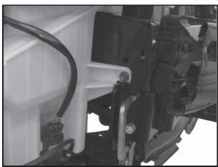
11. On passenger's side, push baseplate up and temporality clamp in place. Now install short rear brace on passenger's side and long rear brace on driver's side, using four 3/8" x 1" bolts, four 3/8" lock washers, and four 3/8" hex nuts. NOTE: Braces attach to bottom hole in baseplate and frame hole hanging from frame. Use "LOCTITE. " blue on all bolts. Do not tighten yet.
