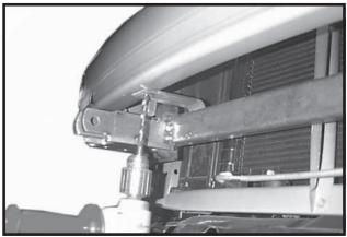
**13.** Drill 3/8" hole through bottom of bumper, using base-plate as template. This is located under bumper on passenger's side.
