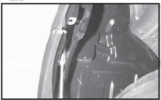
**4.** Remove one screw from facia to fender on each side and carefully remove facia.
