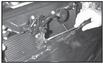
2. Remove one plastic push fastener on top of facia.
