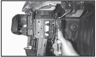
**6.** Temporarily remove two screws from ceramic box and let hang.
