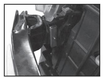
**14.** Install 3/8" x 3-1/2" bolt, 3/8" lock washer, and install through base plate frame, and thread into threaded nut plate on inside of frame. Do not tighten yet.
