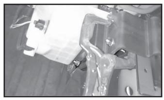
9. On passenger's side, push baseplate up and temporality clamp in place. Now install short rear brace on passenger's side and long rear brace on driver's side, using four 3/8" x 1" bolts, four 3/8" lock washers, and four 3/8" hex nuts. NOTE: Braces attach to bottom hole in baseplate and frame hole hanging from frame. Use " LOCTITE." "blue on all bolts. Do not tighten yet.
