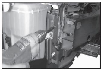
**10.** On passenger's side, drill top hole of baseplate using 3/8" drill bit, using baseplate hole as template. This hole must line up with hole on inside of box frame.
