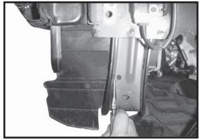
**8.** Remove plastic side shields and set aside for later reinstallation.
