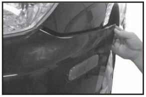
6. Pull facia out at wheel wells and carefully remove facia.
