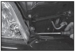
2. Remove three plastic push fasteners on top of facia.
