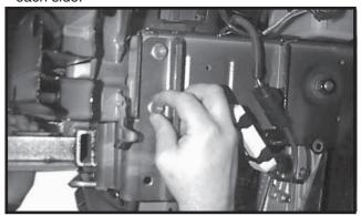
**8.** Slide baseplate up from bottom. On driver's side, start two bolts that were removed from tow eye bracket.
