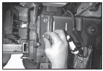
**12.** Slide baseplate up from bottom. On driver's side, start two bolts that were removed from tow eye bracket.
