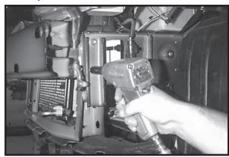
**5.** On driver's side, remove two bolts holding tow eye bracket, these bolts will be reused, bracket will not.
