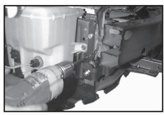
**12.** Next, drill 3/8" hole, using baseplate as template, through flange on vehicle. Install 3/8" x 1" bolt, 3/8" lock washer, and 3/8" hex nut through drilled hole. Tighten all bolts before proceeding. **NOTE:** Use bolt torque chart on front.
