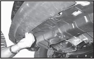
**3.** Remove fasteners from front of belly pan to bottom of facia.
