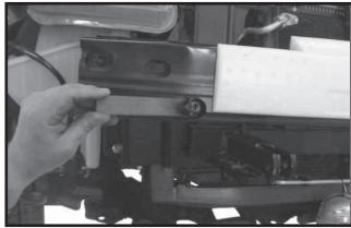
**17.** Slide short nut strip into hole in bumper and use 3/8" x 1" bolt and 3/8" lock washer and tighten bolt.
