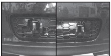
**20.** Cut facia according to picture on each side. Reinstall facia and hardware.
