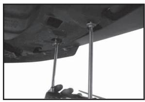
3. Remove eight fasteners from front of belly pan to bottom of facia
