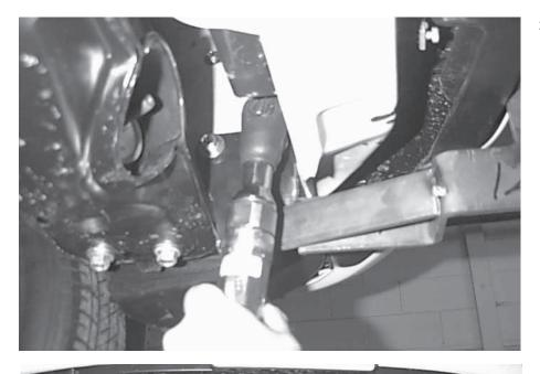
2. Attach right and left mounting bracket with two previously existing bolts on each side.
