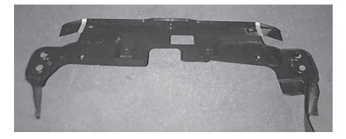
5. Trim splash shield according to photos and install. Note: Lower photos show where ears of splash panel will have to be trimmed off.
