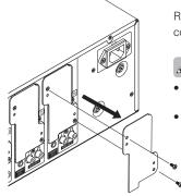
Remove the two screws fixing the cover, then remove the cover.
