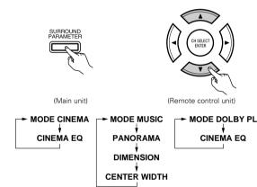
\*\* When set with the on-screen display using the remote control unit while in the MUSIC mode, set the " $\blacksquare$ " mark to "OPTION  $\blacktriangleleft$ " using the  $\triangle$  and  $\nabla$  cursor buttons, then press the  $\triangleleft$  cursor button. Press the ENTER button to return to the previous screen.
