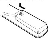
② Set three R6P/AA batteries in the battery compartment in the indicated direction.
