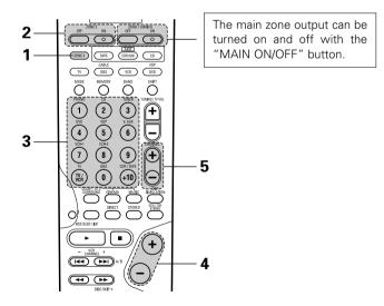
When the ZONE2 SOURCE function is set to TUNER, the preset channel can be selected using the CHANNEL + and - buttons on the remote control unit.
