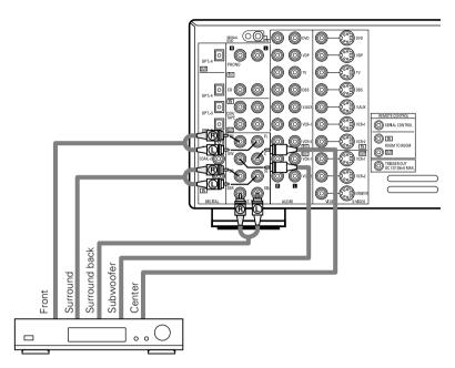
Decoder with 8- or 6-channel analog output
