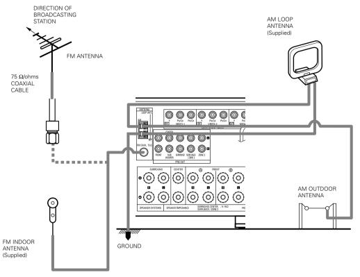
• An F-type FM antenna cable plug can be connected directly.
