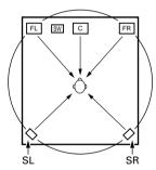
In this case the speakers should surround the listener from all sides to create a uniform sound field from 360°. Ideally the surround speakers should function as "point" sound sources in the same way as the front speakers.
