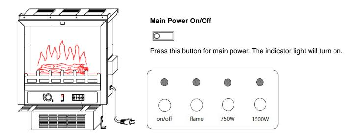
1. ON/OFF Button: Main power and flame effect. The red indicator light will turn on when heater is on.
