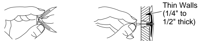
Figure 4 - Folding Anchor Figure 5 - Popping Open Anchor Wings For Thin Walls
