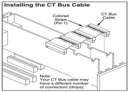
boards in a system. See the *CT Bus/SCbus Adapter Quick Install Card* for installation details about the Adapter and the bus cables. Contact your sales representative to order an Adapter.
