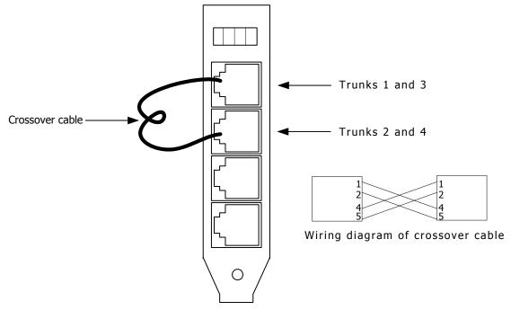
The crossover cable connects the transmit signals from one trunk to the receive signals on another trunk by connecting the pins as shown.
