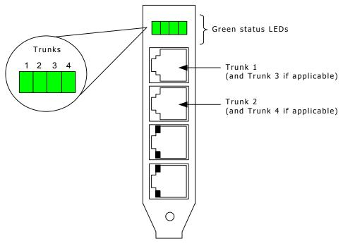
The TX 4000 board end bracket has one green LED for each trunk. The trunk LEDs provide the following indications:
