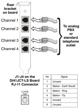
**Note:** Connect the Earth Recall signal to pin 2. DO NOT connect Tip or Ring lines to pin 2 or improper operation of the D/41JCT-LS will result.
