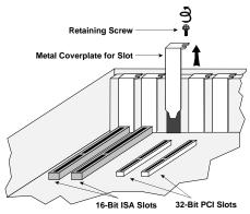
Note: If you are not installing your board in an ISA form-factor PCI slot, remove the slot retainer bracket from the end of the board before installation.
