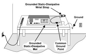
The work surface drains electrical charges from conductive materials when the materials are placed on the surface. The grounded, static-dissipating wrist strap drains static charge from the person wearing the strap. Both components ensure that static charges are drained at a rate and current level that are safe. Both must be used any time a person is handling a board or component.
