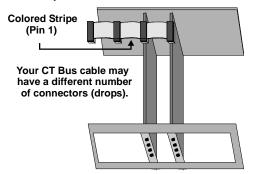
3. If the cable has extra connectors or is loose, tuck the cable down so that it does not snag when you replace the computer cover. See the **Caution** given earlier in this section.
