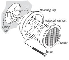
speaker wires through tweeter cup, connect tweeter to wires, and snap tweeter into cup by aligning the notches. Be careful not to push on the center of the tweeter grill.
