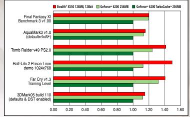
\*Radeon X550 128MB 128-bit compared with GeForce<sup>™</sup> 6200 with 256MB TurboCache<sup>™</sup> and GeForce 6200<sup>™</sup> 256MB. Test system Intel Pentium 4, 3.4GHz, 512 MB RAM. Graphics settings: 1024x768. Drivers: ATI 8.121rc1, NVIDIA 71.84.
