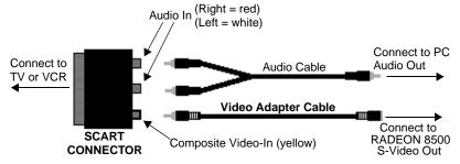
The above illustration shows how to connect your RADEON 8500 to a European TV using the SCART.
