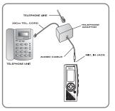
CONNECT LINE-IN CABLE TO THE MICROPHONE JACK ON THE VOICE RECORDER AND TELEPHONE ADAPTOR. CONNECT TELEPHONE CABLE TO TELEPHONE ADAPTOR. PRESS "REC" BUTTON FOR RECORDING. IF YOU SET UP THE "ARS", AUTOMATICALLY START RECORDING IF THERE IS ANY SOUND AND PAUSING IF THERE IS NO SOUND.
