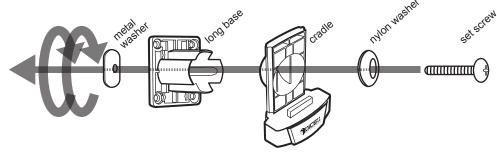
If the long base will fit your car interior more appropriately than the short one, then please follow the illustration to attach the long base to the cradle. Turn the base clockwise to tighten the base to the cradle.
