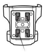
These holes are designed to fit vehicle mounts from iGrip™
