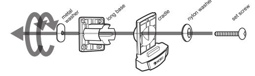
If the long base will fit your car interior more appropriately than the short one, then please follow the illustration to attach the long base to the cradle. Turn the base clockwise to tighten the base to the cradle.
