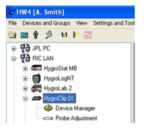
To open the Device manager form, click with the mouse on Device Manager. The Device Manager form is used to configure the HygroClip DI and to read device specific information. When Device Manager is started, it automatically interrogates the device and downloads its current configuration.
