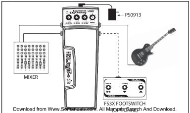
Connections Diagram - Flexible Output Mode 3 (Stereo Amp)
