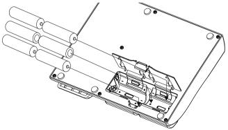
Connecting a cable to the Input applies power to the RP80. Disconnecting your instrument from the Input of the RP80 disconnects the battery power. Turn your amplifier(s) on and adjust the volume(s) to a normal playing level. To prolong the battery life, disconnect your instrument from the RP80's Input when not in use .
