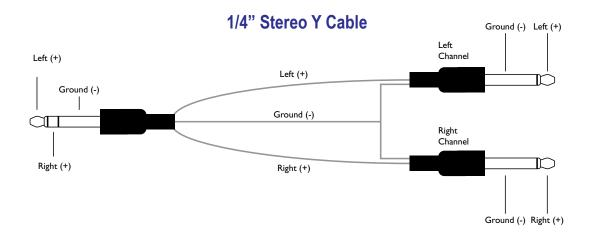
**NOTE:** The 1/4" Output must be configured for stereo operation for this type of setup. See "Mono/ Stereo Operation" on page 21 for more information.
