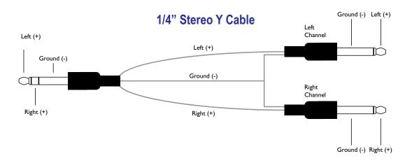
**NOTE:** The 1/4" Output must be configured for stereo operation for this type of setup. See "Mono/ Stereo Operation" on page 21 for more information. When connecting directly to a recording device, SCC must be enabled. See "Speaker Cabinet Compensation (SCC)" on page 21 for more information.
