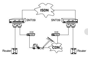
The routing on an alternative connection takes place **without interrupting the data transmission**, therefore each terminal connected to SNT09 can "see" the geographic connection in a **transparent** way.
