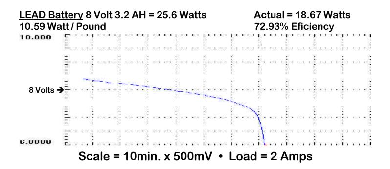
As you can see the Digital Camera Battery provides steady power from start to finish. The unregulated output from other packs can cause over voltage and brown out conditions that can damage sensitive electronics. The unregulated output of the LEAD cell and many other types of rechargeable packs can also provide very high currents that could start an electrical fire in a matter of seconds if the cable should become shorted or damaged.
