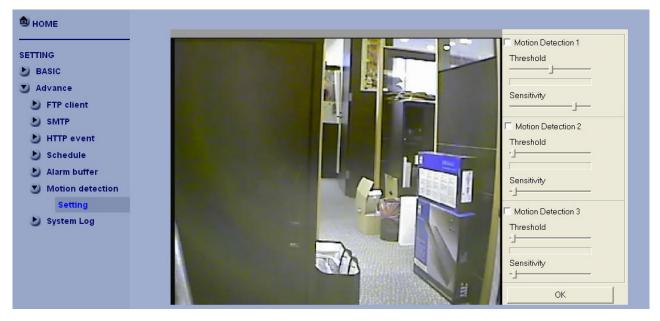
Click it On when you use the Motion Detection function and detecting zone appears for adjusting and moving. The common setting options are displayed below. If you do not wish to use the Motion Detection function, click it Off and press OK.
