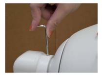
• unscrew the bottom screw to install cables.
