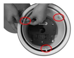
Finally cover up the smoked cover to accomplish the installation. Please be sure hands are clean while cover up, or it may dirty the cover. It's recommended to tear off the protect membrane after installation is finished, or wear on gloves.
