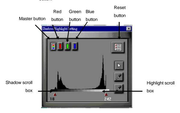
You will see a graph representing the intensity of the tones in the image. Below the graph is a scroll bar with one scroll box at each end. The box on the left is the Shadow scroll box; the one on the right is the Highlight scroll box.
