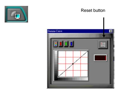
A graphical mapping of the gamma curve is displayed.
