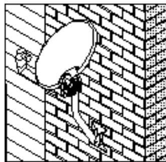
Installing the satellite dish antenna on a brick surface. See the section titled "Installing the Satellite Dish Antenna Onto a Brick Surface."
