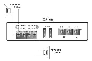
Note that the two speakers & four speakers have been connected to the four terminal following the (+) and (-) graphic. Your speaker terminal may be marked (+) and (-) or there may be red dot by one terminal which means the same as (+).
