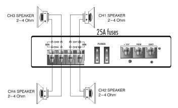
Note that the two speakers & four speakers have been connected to the four terminal following the (+) and (-) graphic. Your speaker terminals may be marked (+) and (-) or there may be red dot by one terminal which means the same as (+).
