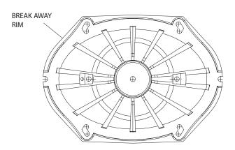
The model SX570 speaker has a break away rim to facilitate mounting as either a 6 X 8 or a 5 X 7 speaker. The mounting size required varies depending on the vehicle manufacturer.
