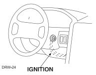
Once the lower dash panel has been removed, locate the ignition harness at the back of the key cylinder. This is usually a group of thicker wires. With the ignition harness exposed, use your digital multi-meter to find your power and ignition wires.
