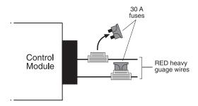
Once the constant power wire has been identified, solder the two thick RED wires from the control module to it and cover the connection with electrical tape to ensure a safe connection.
