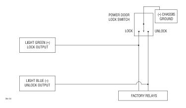
Once the correct wire has been found, solder the small LIGHT GREEN wire off the main connector to it and cover the connection with electrical tape.
