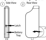
1. Using a small flat narrow object, push latch down towards battery tray while gently prying the tray outwards from both ends until released. Remove the tray from the remote control housping.
