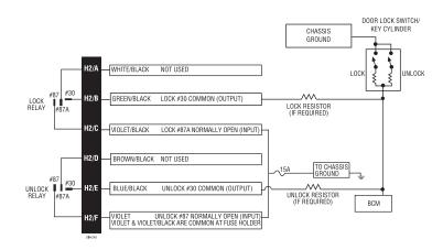
Locate the suspected lock wire, and with the red meter lead still secured to a (+)12 volt source, probe the suspect wire with the black lead of the meter. Press the door lock switch to the lock position and watch the meter display. The correct wire will show a 10.00 to 12.00 volt pulse when the switch is pressed.
