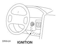
Once the lower dash panel has been removed, locate the ignition harness at the back of the key cylinder. This is usually a group of
