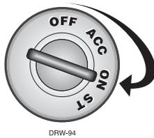
To disarm the security system, turn the ignition to the ON position. Press the Valet button the preset number of times (one to
