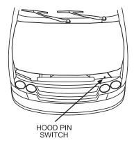
Installing the hood pin switch requires drilling a ¼-inch hole in the metal lip under the hood. Choose a location that will allow the pin switch to be depressed when the hood is closed. The pin switch has a spade connector on the bottom for the wire connection.
