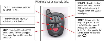
N.B.: Pressing the LOCK and UNLOCK buttons simultaneously will activate the AUX 2 output.
