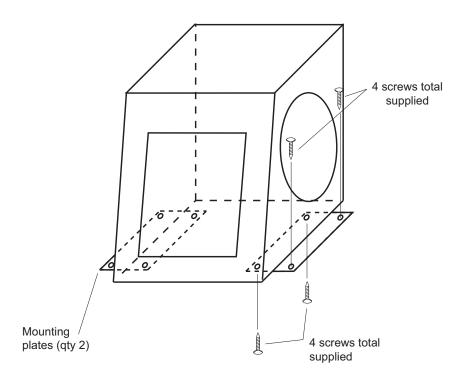
Note: The mounting plates can be installed on any edge of the bottom surface of the subwoofer (shown above mounted on the left and right).
