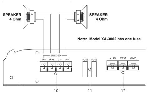
For bridging into a single speaker load, the XA-3002/6002 have the ability to be bridged, as shown in the diagram below:
