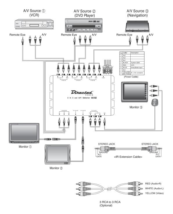
**NOTE:** The BLUE wire of the Power Harness connects to the emergency brake. All A/V outputs are **enabled only when this wire is grounded**.
