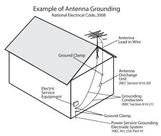
Do not locate the antenna near overhead light or power circuits, or where it can fall into such power lines or circuits. When installing the antenna, take extreme care to avoid touching such power lines or circuits, as contact with them can be fatal.
