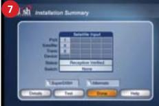
This should clear out any previously installed devices. Then, select **Done**.
