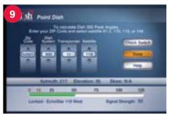
Once accurately pointed, the signal meter will turn green. Make small adjustments to get the signal as high as possible. Check that the bar at the bottom of the screen is green
