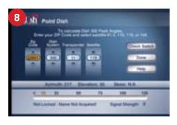
Input zip code of current location and dish type. Zip Code should be the zip code of your current location. Note that whenever you move the satellite antenna to a new location, you must enter the zip code of your new current location.
