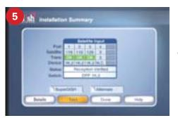
If your receiver is showing a switch type of DPP1K.2, then a check switch test is not necessary. In that case, skip to step 7 to complete DISH receiver setup.
