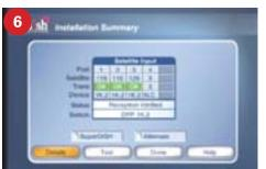
Verify that the check switch resulted in a switch type of DPP 1K.2 and that there is a green OK status on Satellite 110, 119 & 129.
