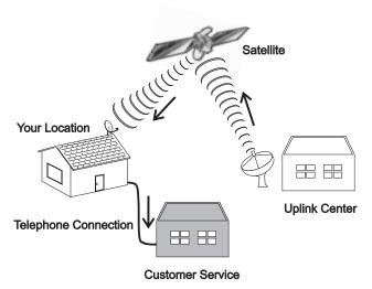
place on the surface of the Earth. Once the satellite dish is aimed at the satellite, the dish does not have to move to follow it.
