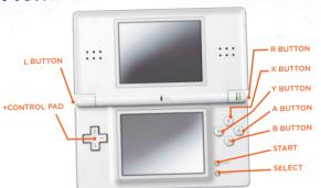
Use the **Touch Screen** and **stylus** to select and choose items on the menus. You can also use **+Control Pad** and the **A** and **B Buttons** to get around the menus.
