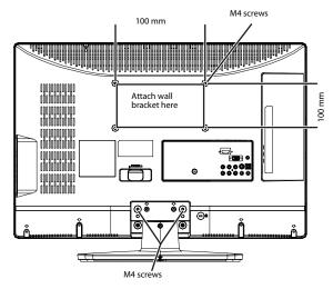
**2** Remove the scew from the bottom of the base.
