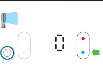
Press the blue thermostat control button to change the target temperature to 0°C. The power button light will change from red to blue. To adjust the airflow speed use the airflow speed control.
