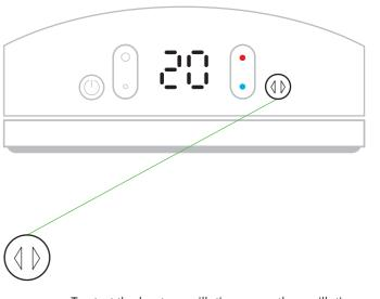
To start the heater oscillating, press the oscillation control button. The heater will not oscillate when the control buttons are pressed.
