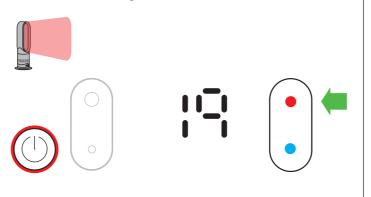
Press the red thermostat control button until the digital display shows the desired target temperature. The power button light will change from blue to red.
