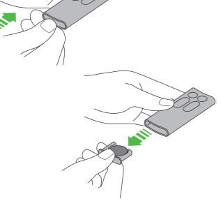
Press the end of the remote to release the battery.
