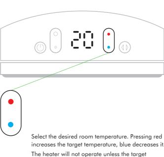
increases the target temperature, blue decreases it. temperature is above the room temperature.
