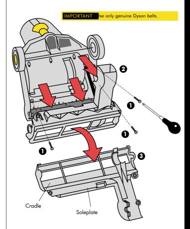
3 If cradle becomes detached from soleplate, align circular ends of cradle with corresponding holes of soleplate and slot into place, ensuring that 'front' edge of cradle faces the right direction.
