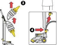
Remove clear bin and cyclone top, by lifting up until it releases. Then gently pull off from ball socket.
