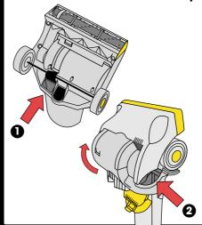
Turn machine upside down. Remove soleplate. Raise inspection flap and look down through aperture. If you cannot see daylight, remove any blockage with a stiff wire.
